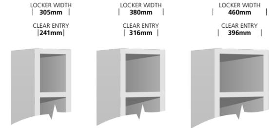
Allow up to 2.5mm per locker for horizontal creep
